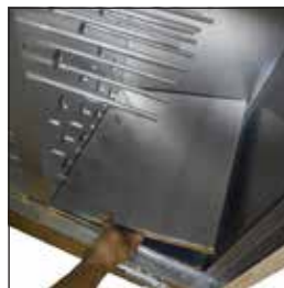
A3. Remove the aluminium panel
